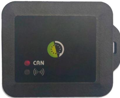
KiwiBridge is a device that acts as a radio bridge between the detection system (Anti-Collision, KiwiEye, Radar) and KiwiSafe, the LED interface in the cab for displaying obstacles.
